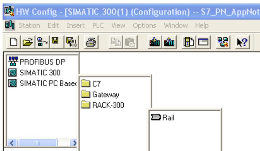
An empty station grid is displayed. The components of the local PLC rack need to be added to the grid, which in this case includes a power supply and the CPU.
