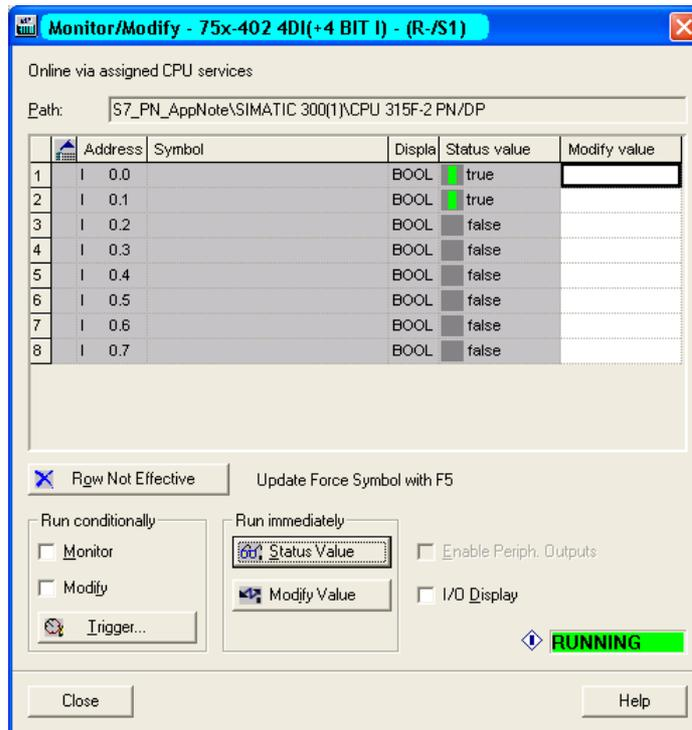
The digital input and output modules are displayed in binary format and analog modules are in word format.
