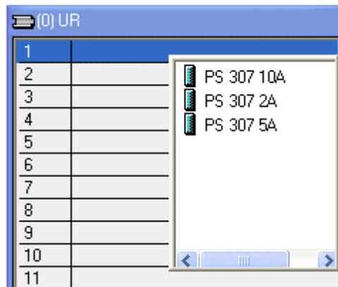
Right-click on Slot 2 and select **Insert Object...**. Then select the model and version of the CPU.
