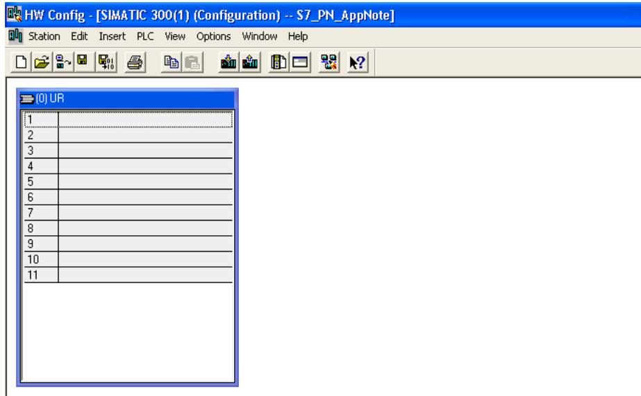
Right-click on Slot 1 and select **Insert Object...**. Then select the power supply for your system.
