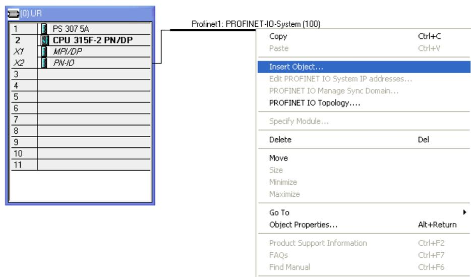
From the menu, select **Additional Field Device**. A list of installed devices is displayed. Select the **750-340 V01.00.xx**.
