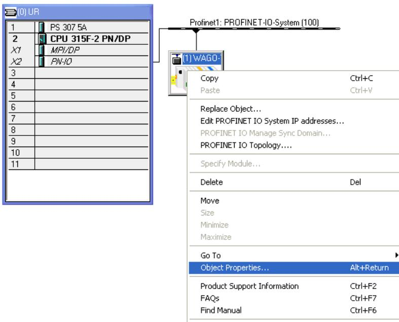
A *Properties* dialog box is displayed. The default Device Name and Device Number are displayed for the WAGO 750-340. The STEP 7 HW-Configuration automatically generates these values from the device profile. These values can be change if desired. Click **OK** to continue.
