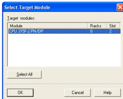
Select the device type from the *Target modules* list and click **OK**.
