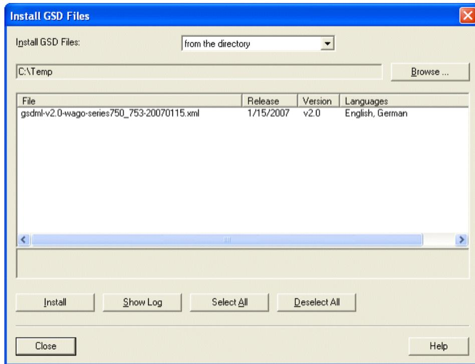
After successfully installing the WAGO 750-340 GSD file, its profile is available for the STEP 7 HW-Configuration tool.
