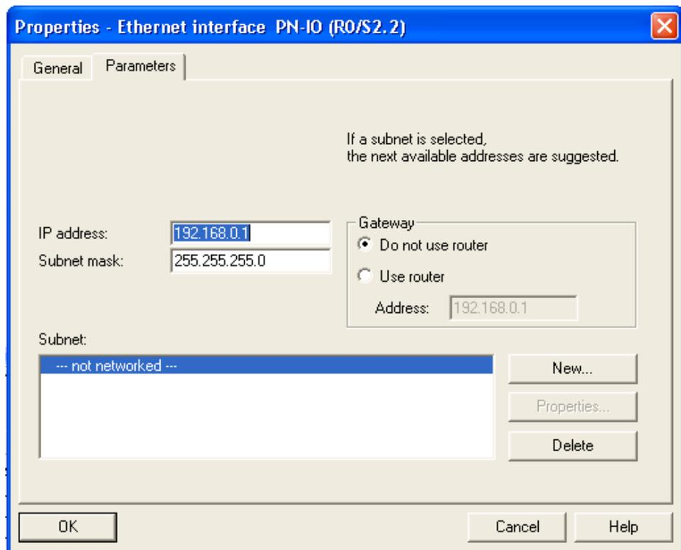
Another *Properties* dialog box is displayed for defining a new subnet. Enter a name for the PROFINET network, such as **ProfiNet1** and click **OK**. Click **OK** a second time to exit the *Properties* window.
