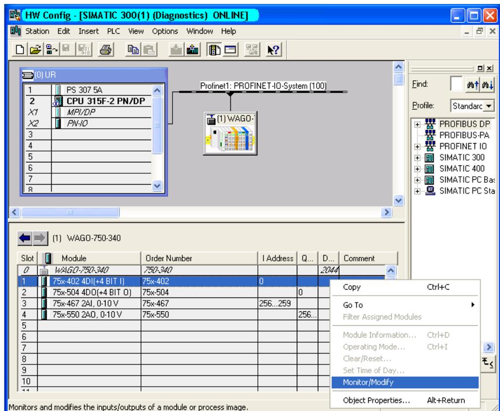
The *Monitor/Modify...* dialog box displays the inputs of the 750-402 module in table format. Click on the **Status Value** button to refresh the screen.
