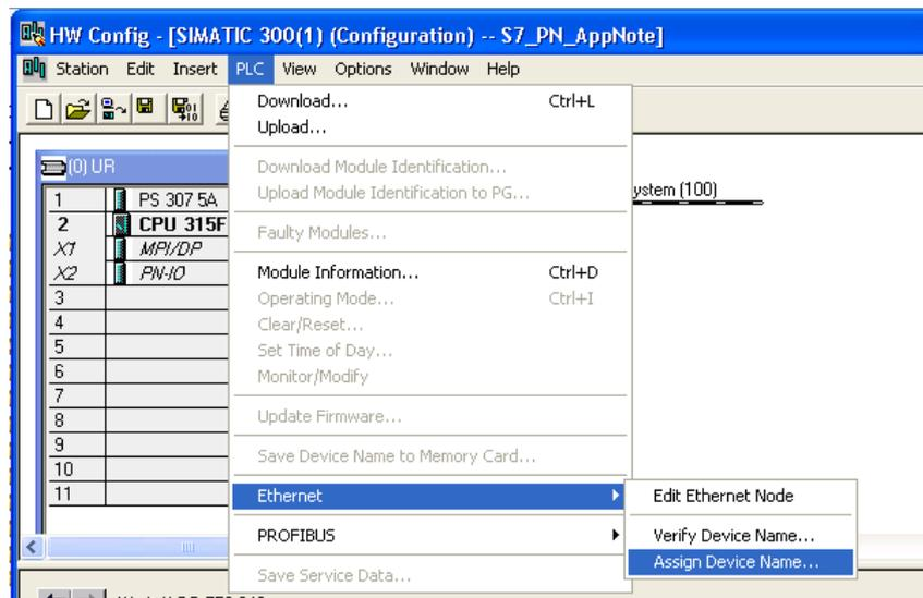
The device name for the selected WAGO 750-340 node is displayed in the *Device name* list box (in the example below the device name is also called “WAGO 750-340”). To assign this configuration to a physical device, select the physical device from the *Available devices* list, and click the **Assign Name** button.
