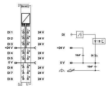
Figure 6: Schematic diagram
