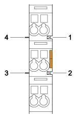
Figure 3: Power Jumper Contacts
