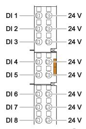
Figure 4: CAGE CLAMP® S Connectors
