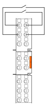
Figure 11: Connection Example with 2 Switches on Channel 1 and 2
