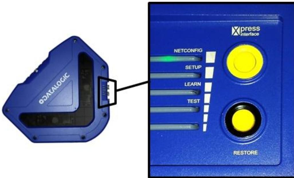
Figure 43: Control Panel Buttons
