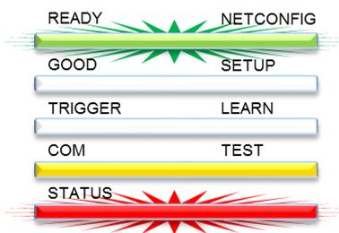
**STATUS/READY + COM = Laser Failure**
