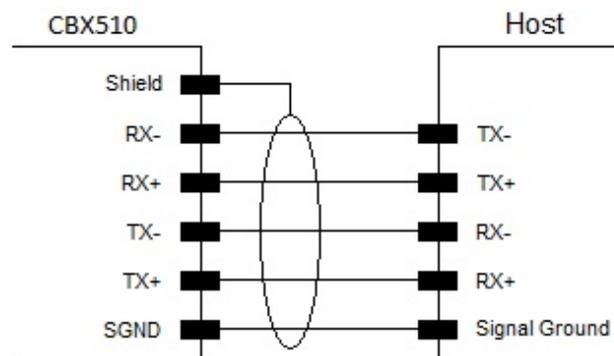
Figure 28 - RS422 Full-Duplex Interface Connections: Host – CBX510
