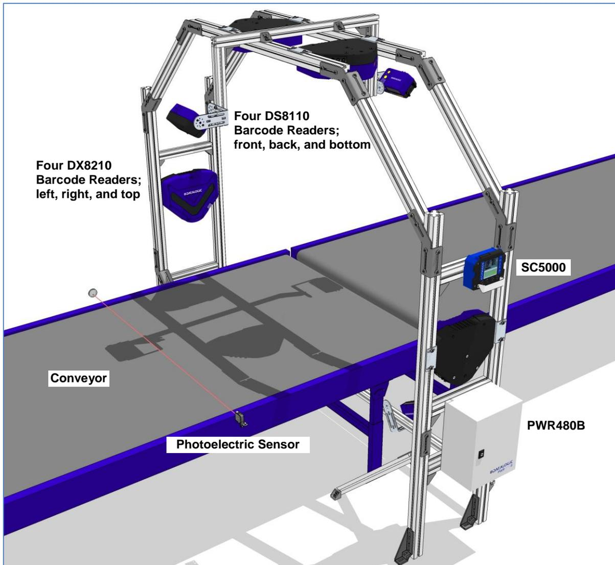
Figure 73 – Example Large Synchronized Network Reading Station
