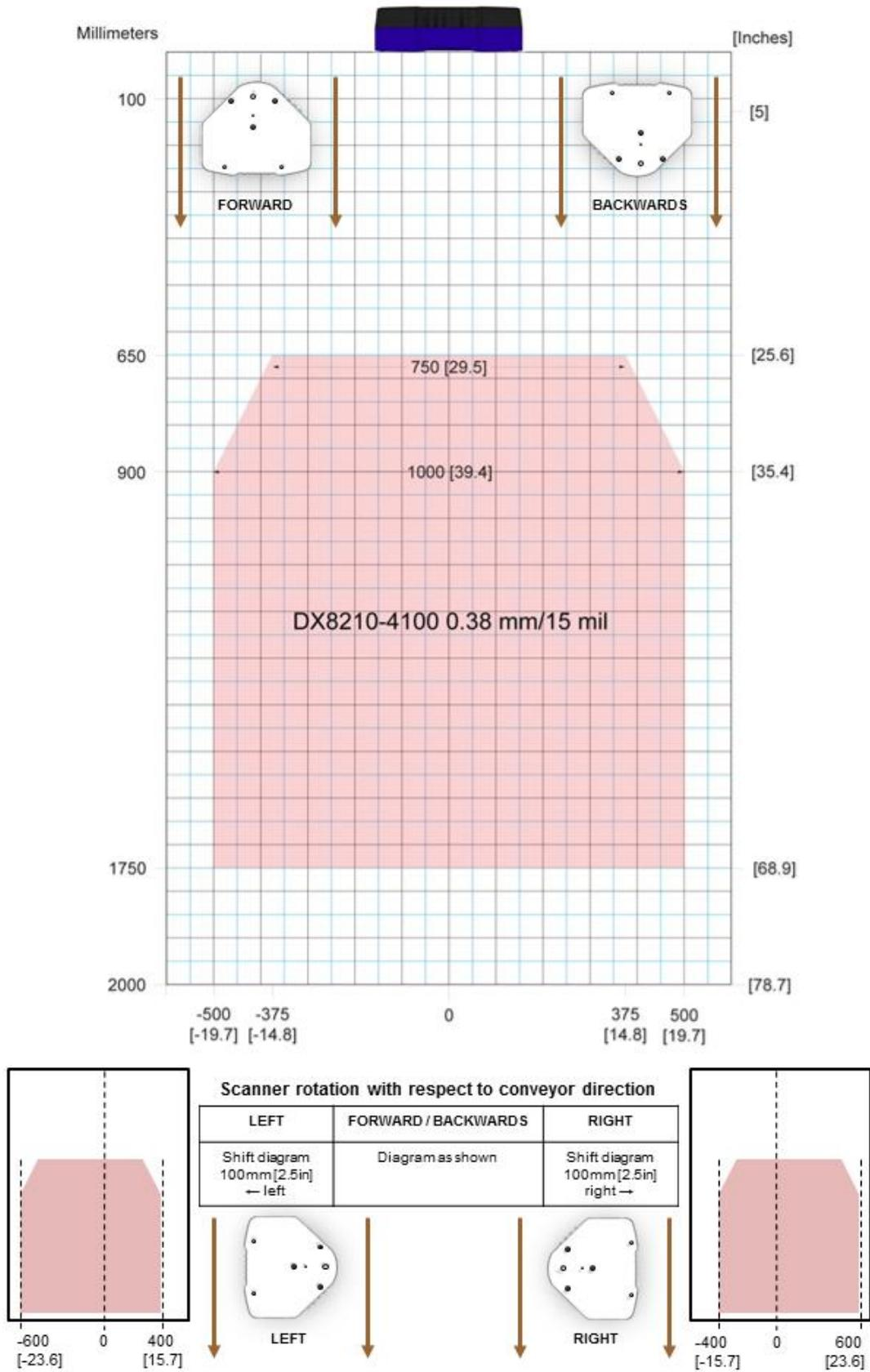
Figure 85 – Reading Diagram for DX8210-4100 0.38 mm/15 mil
