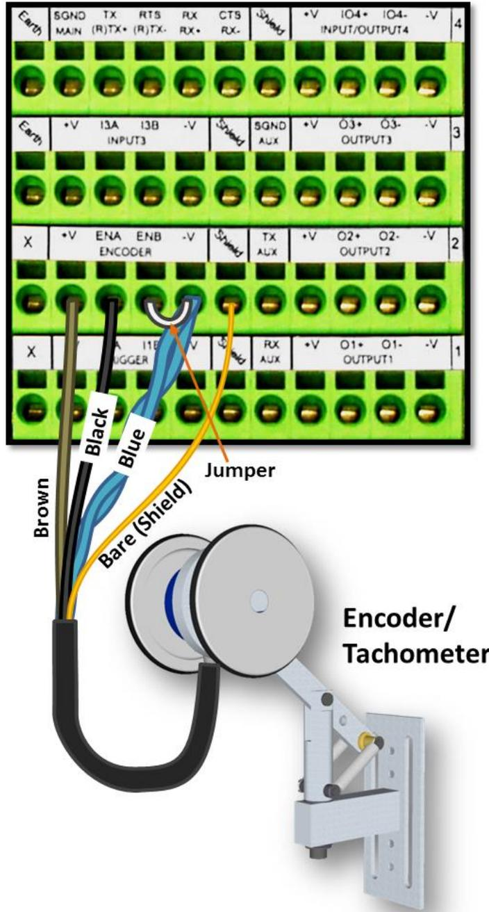
Figure 35: OEK-4 (95B082050) Encoder/Tachometer Wiring (PNP Output)
