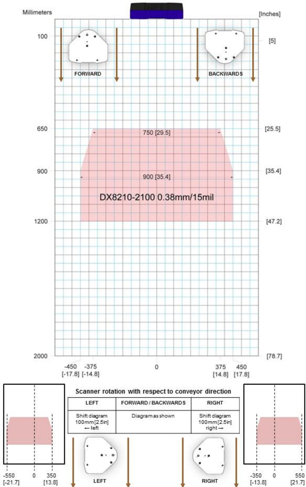
Figure 83 – Reading Diagram for DX8210-2100 0.38 mm/15 mil
