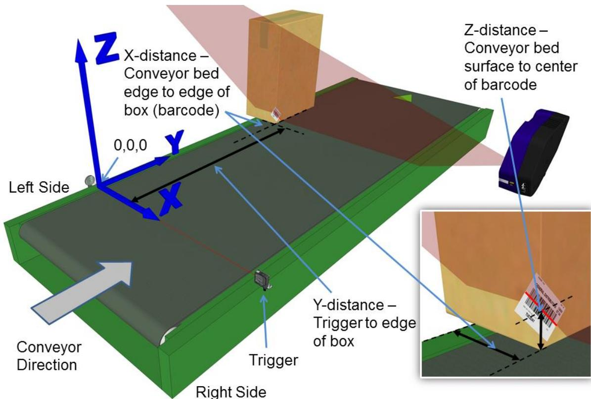
Figure 62: Side-read 1<sup>st</sup> barcode placement
