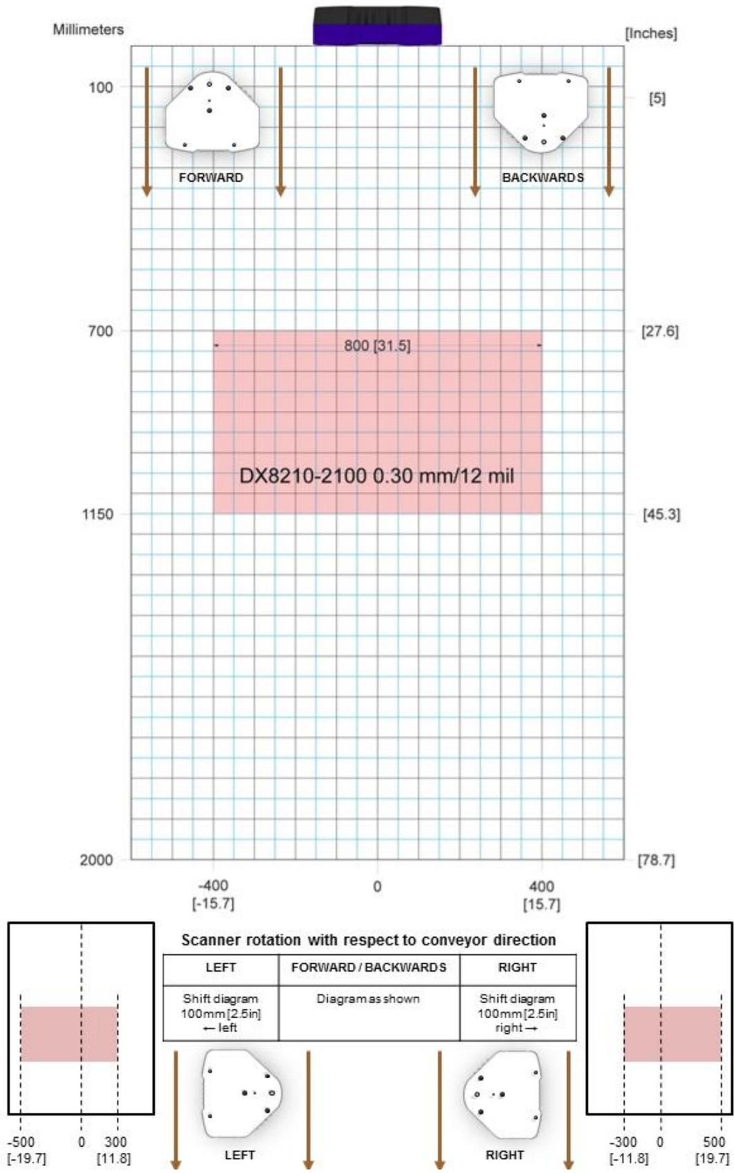
Figure 82 – Reading Diagram for DX8210-2100 0.30 mm/12 mil
