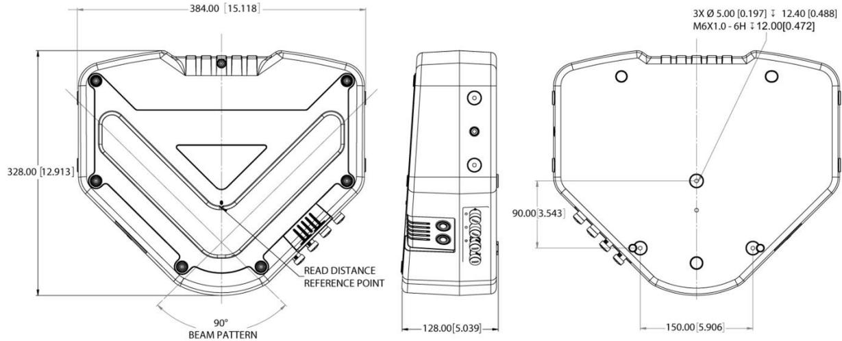
Figure 13: DX8210 Overall Dimensions
