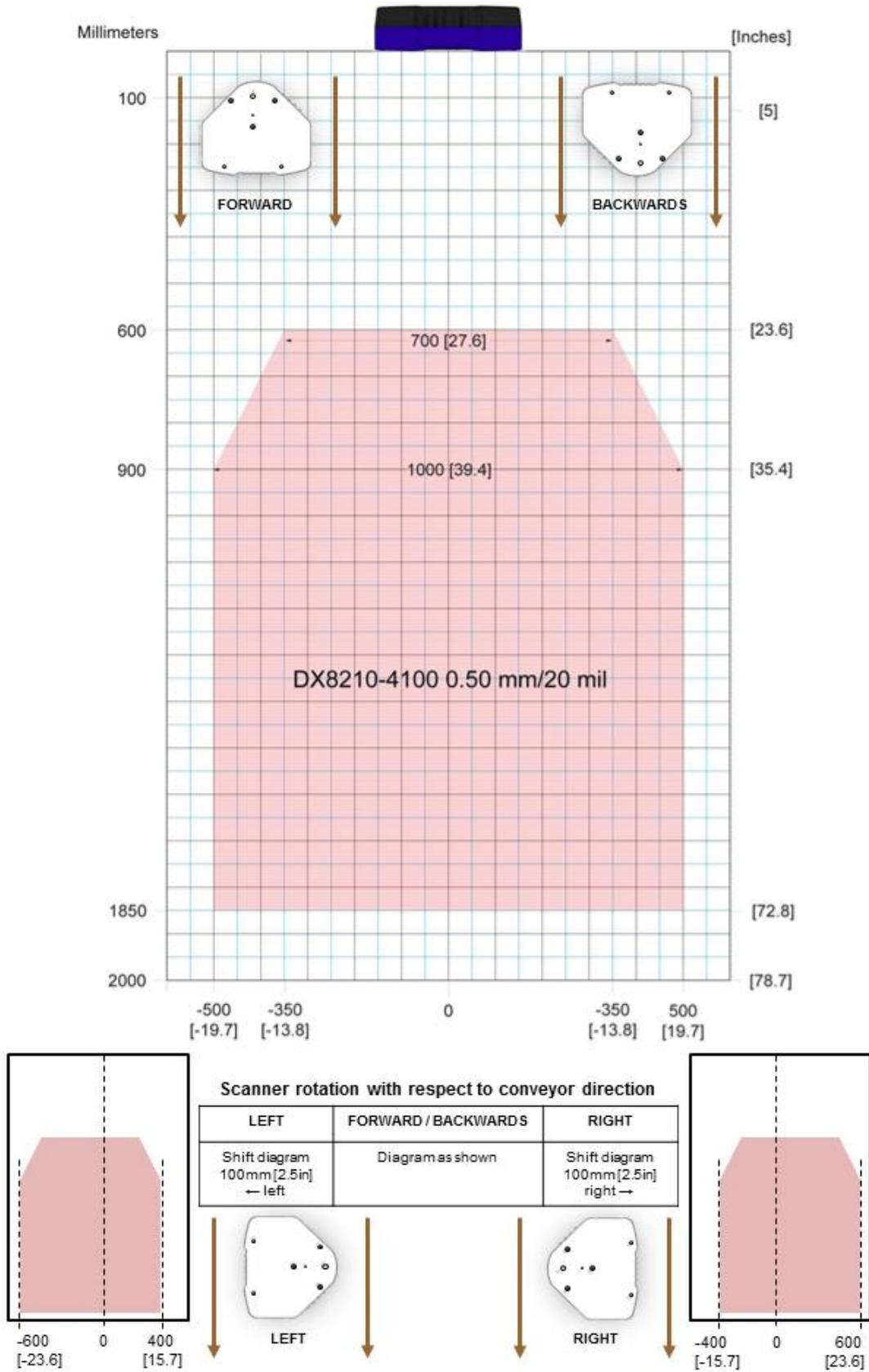
**Figure 86 – Reading Diagram for DX8210-4100 0.50 mm/20 mil**
