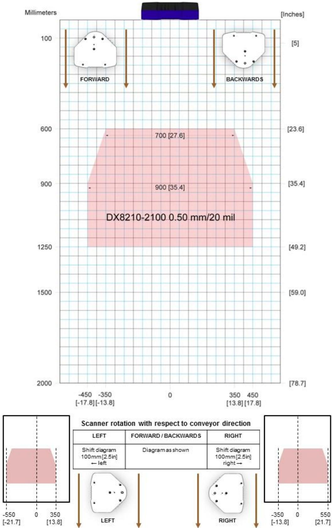
Figure 84 – Reading Diagram for DX8210-2100 0.50 mm/20 mil
