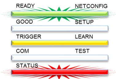
**STATUS/READY + TRIGGER = Motor Failure**
