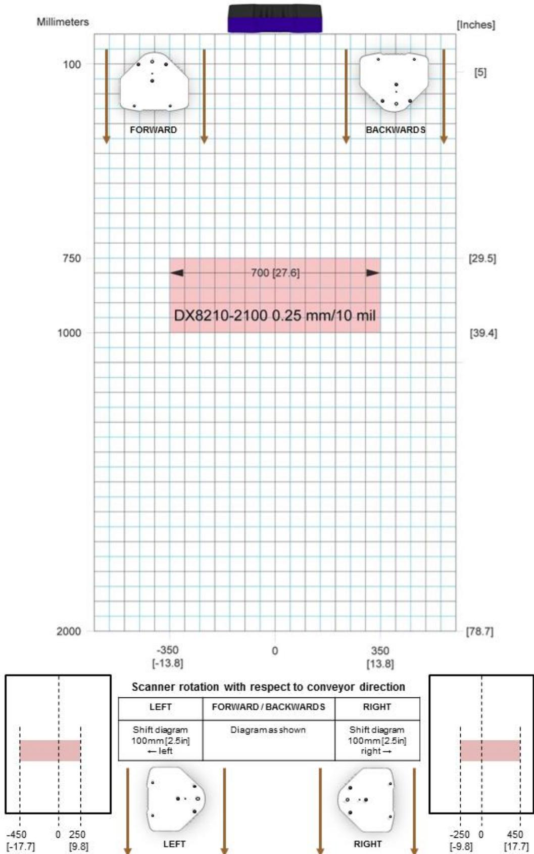
Figure 81 – Reading Diagram for DX8210-2100 0.25 mm/10 mil
