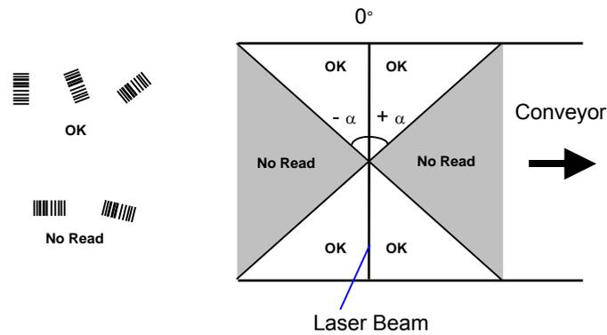
Figure 78 – Reading Zones with  $\alpha$  Max
