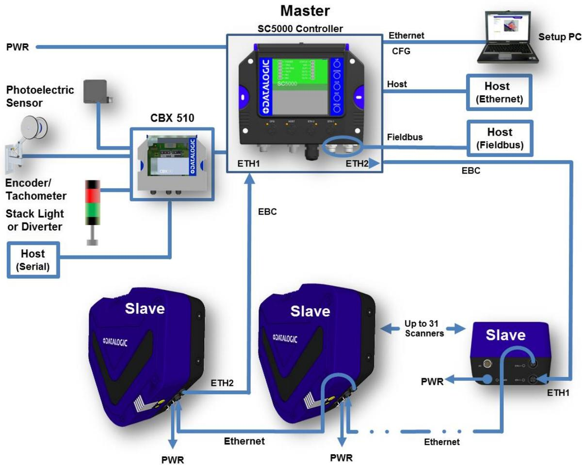
Figure 23: DX8210 Array (Tunnel) to SC5000 (alternate with CBX)
