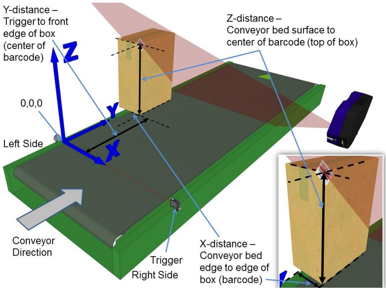
Figure 64: Side-read 2<sup>nd</sup> barcode placement
