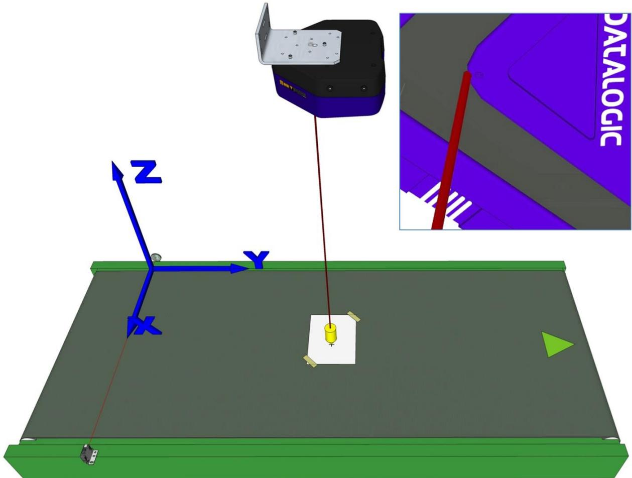
Figure 46: Using a plumb bob to mark scanner location on conveyor
