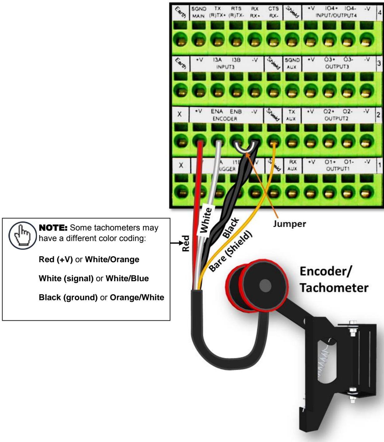
Figure 34: OEK-2 (93ACC1770) Encoder/Tachometer Wiring (PNP Output)
