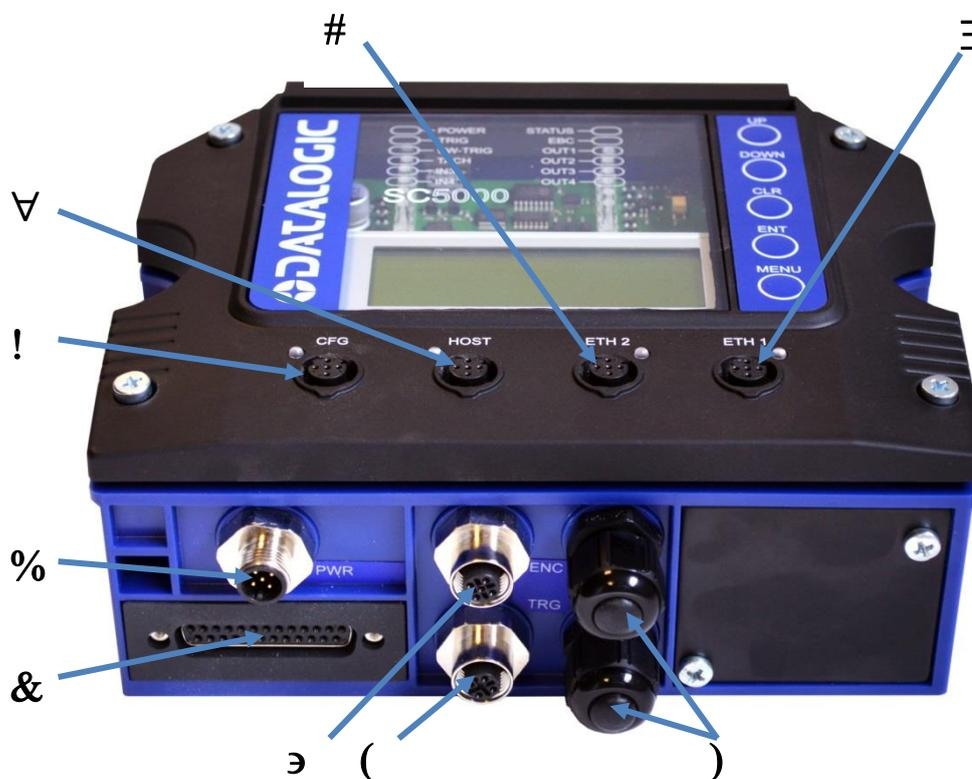
Figure 39: SC5000 Bottom Panel Connectors
