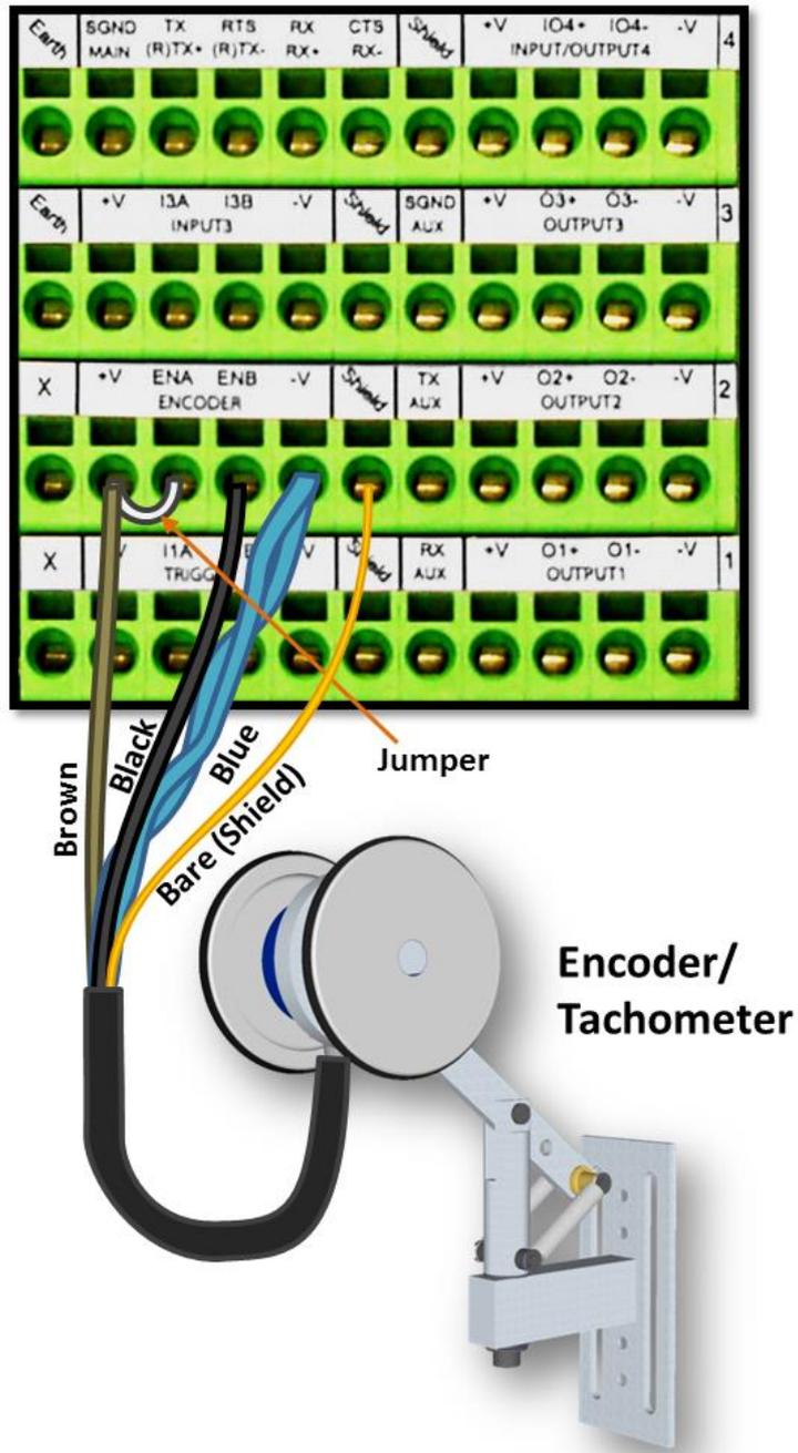
Figure 33: OEK-4 (95B082050) Encoder/Tachometer Wiring (NPN Output)
