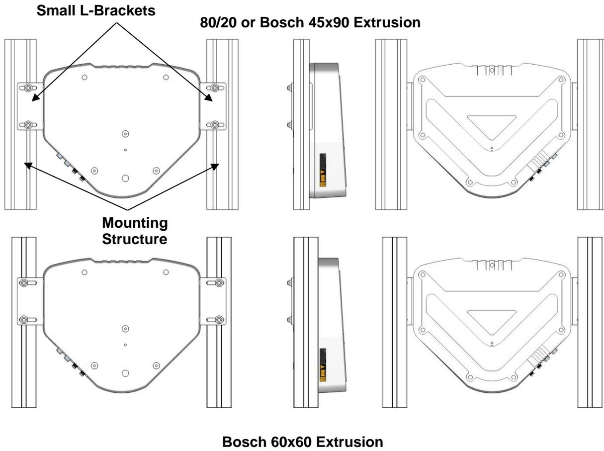
Figure 17: DX8210 Small L-Brackets Mounting Options (93ACC0079)
