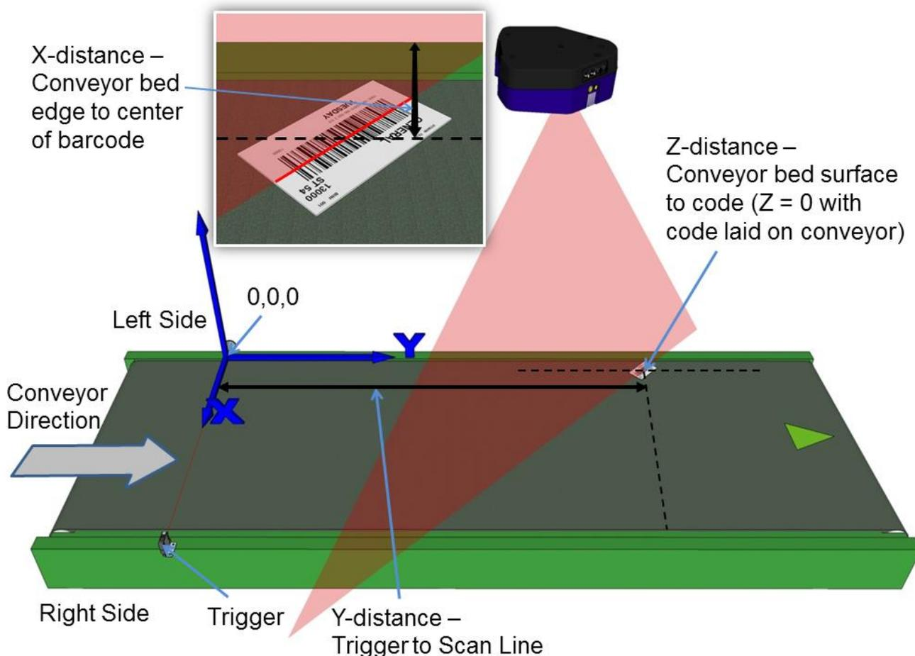
Figure 55: Top-read 1<sup>st</sup> barcode placement
