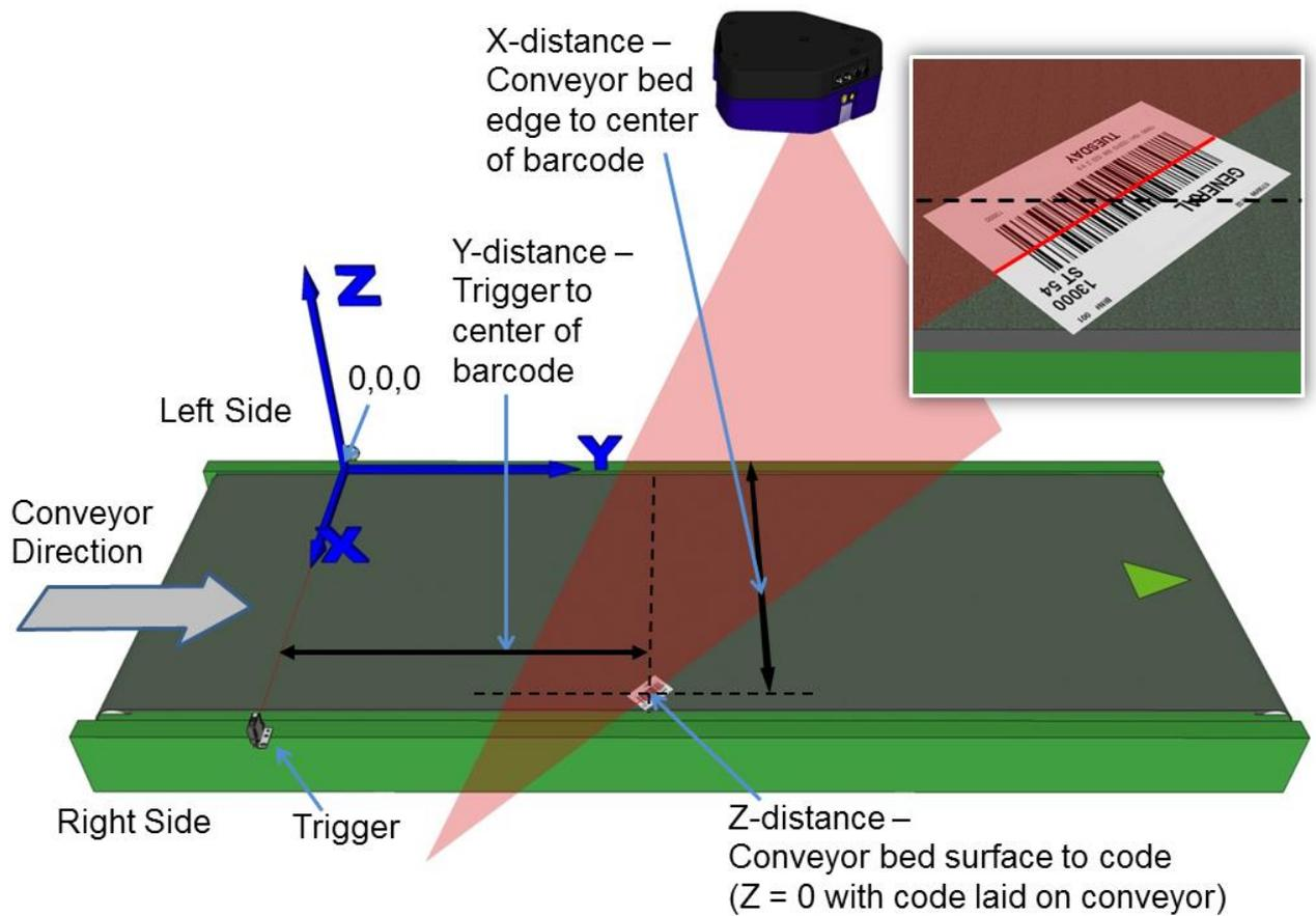
Figure 57: Top-read 2<sup>nd</sup> barcode placement
