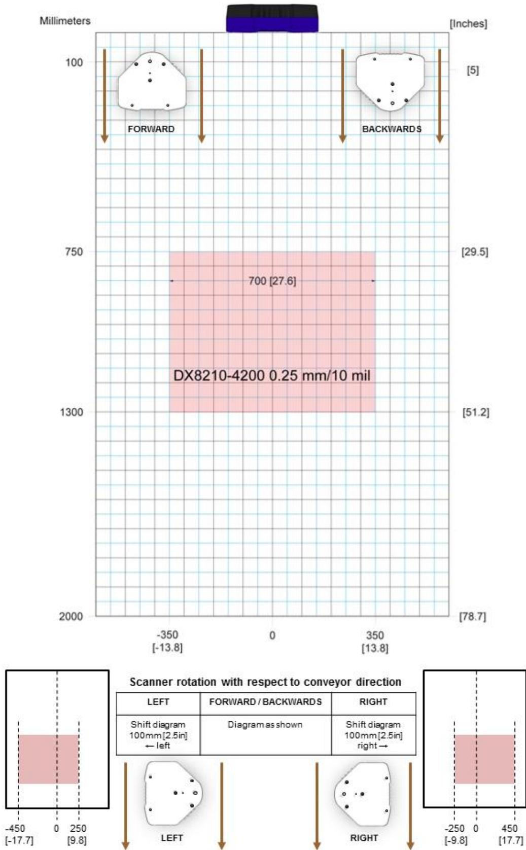
Figure 87 – Reading Diagram for DX8210-4200 0.25 mm/10 mil
