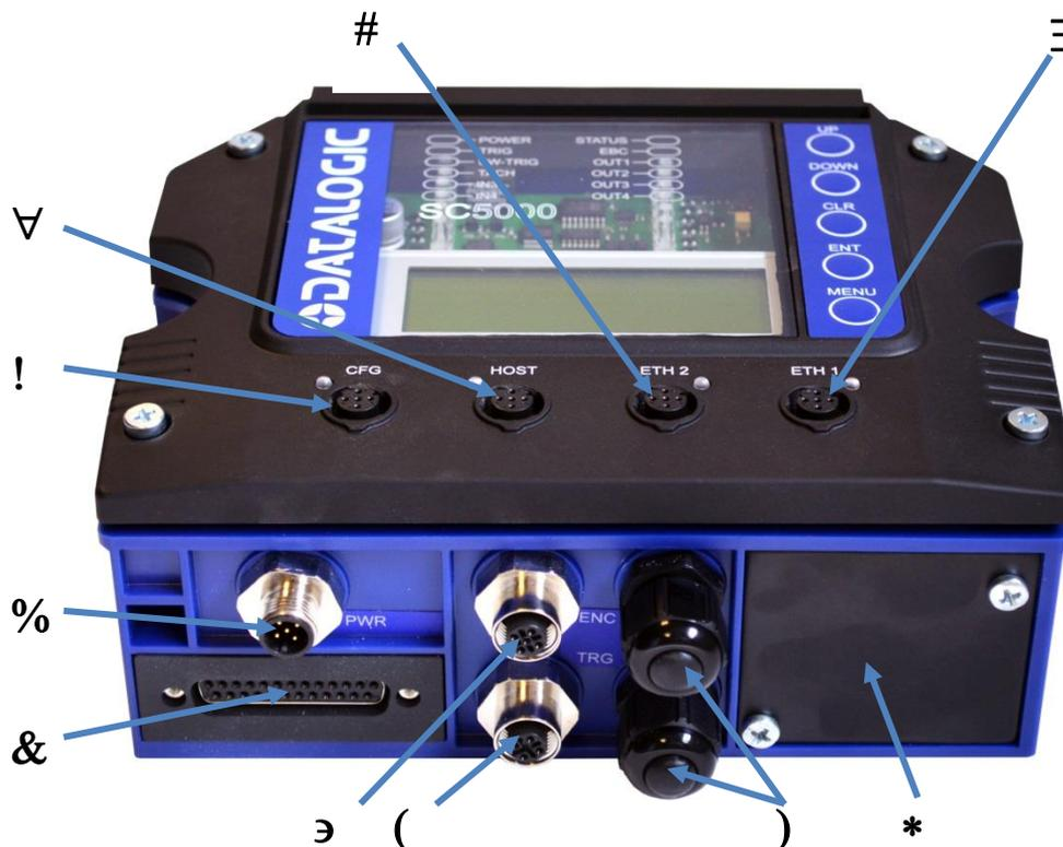
Figure 41 - SC5000 Standard Model Connector Panel
