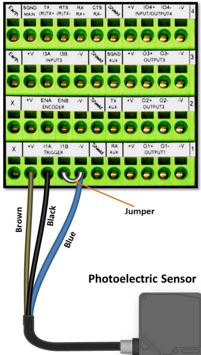
Figure 31: Photoelectric Sensor Wiring (PNP Output)
