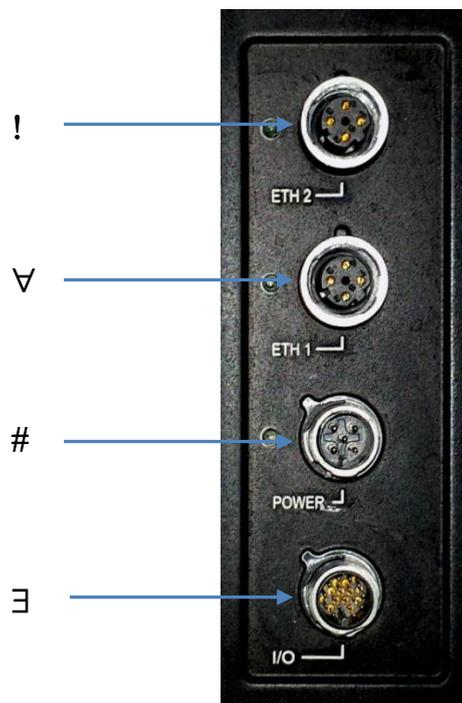
Figure 24: DX8210 Connector Panel
