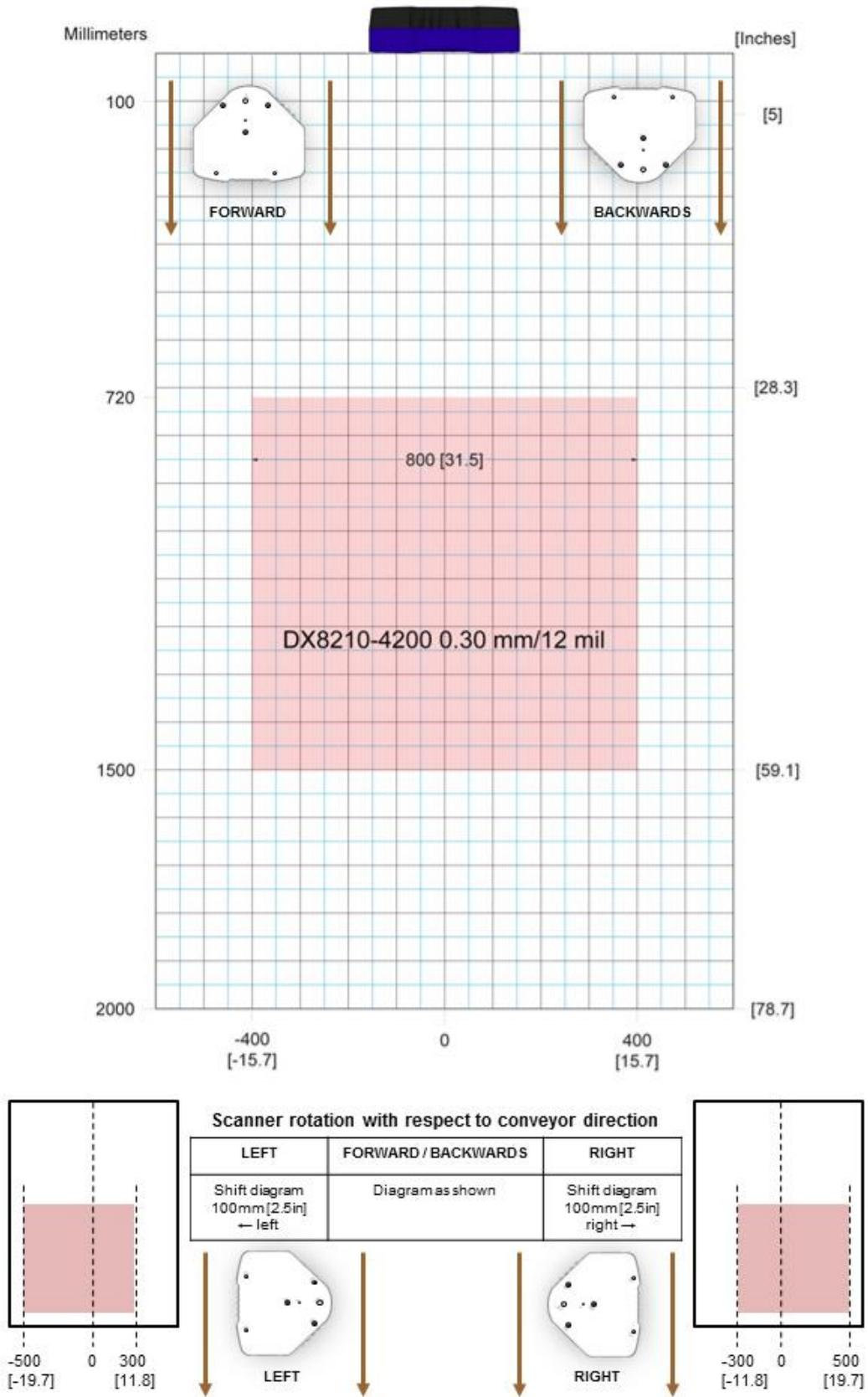
**Figure 88 – Reading Diagram for DX8210-4200 0.30 mm/12 mil**
