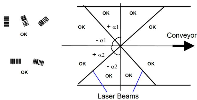
Figure 79 – X-Pattern Reading Zones with  $\alpha$  Max
