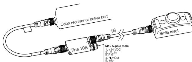
Connection of Smile 11 ROx to Orion through Tina 10B. For connection to Vital control module or Pluto Safety PLC.
