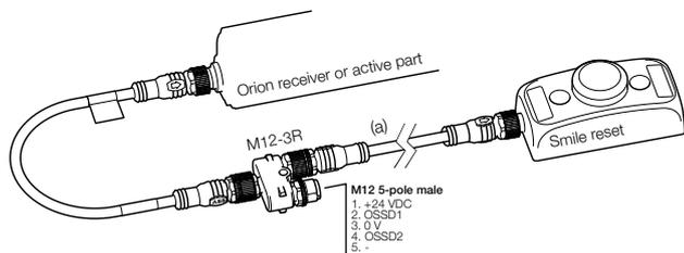
Connection of Smile 11 ROx to Orion through M12-3R. For connection to any control module compatible with OSSD outputs.
