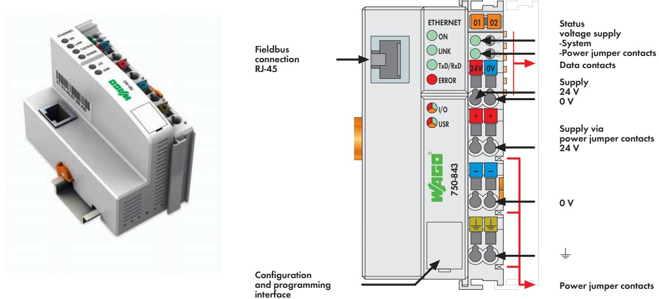
The ETHERNET PLC combines control functionality, I/O interface and ETHERNET in one device.
