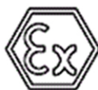
Figure 80: Side Marking Example for Approved I/O Modules According to ATEX and IECEx
