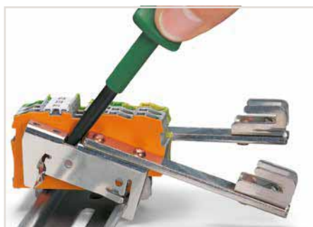
Remove the busbar carrier using an operating tool (type 3, 5.5 x 0.8 mm blade).
