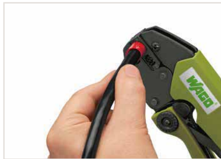
Squeeze handles until ratchet mechanism is released.
