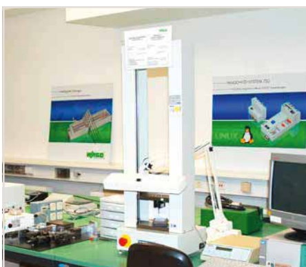
Conductor Retention Force Testing
