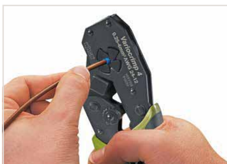
Squeeze handles until ratchet mechanism is released.
