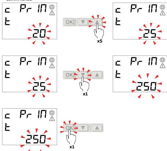
3. Repeat the operations described in steps 1 and 2 until the desired number is obtained, press "OK" to confirm the number.
