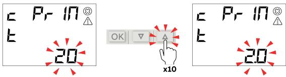
Some device configurations allow entering the comma. Comma can be displayed by increasing the number with " $\mathbf{Up}$ ", after character 9 and before data entry starts again from character 0.
