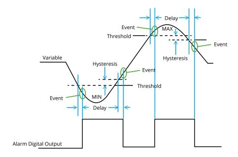
When the value of the alarm variable exceeds the threshold and the delay, the alarm will be generated; and when the alarm variable recovers to the normal range and exceeds the hysteresis and delay, the alarm will be released. Alarm can be connected to certain DO to control the alarm signal output at the DO. If the alarm is stored in flash, it can be viewed later in the read data menu. When the device is in alarm state, ICON will be displayed.
