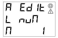
"Edit" indicates that the alarm is already present. If it needs to be modified, press the button "OK" to go to the event and modify the configurations.
