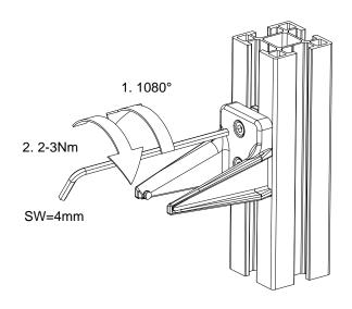
JSM 55 is designed to fit ABB Jokab Safety Quick-Guard aluminium profiles, but can be used on any flat surface.
