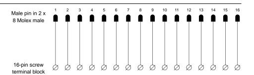
Note: 16-pin screw terminal block with internal connection adapted for a common monitoring unit. Designed for a manually connected cable. Anti-cheat-board is an option.
