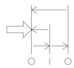
The symbol for the 3-position switch shows the three positions (OFF, ON, OFF) with O and I, actuating force from left to right, and possible paths for the switch (IEC 60947-5-8:2006).
