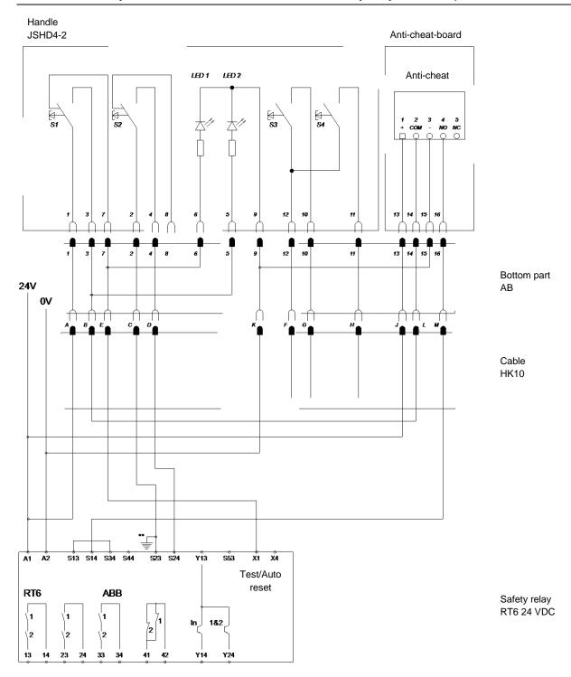
Note: The anti-cheat-board is connected in series with the first 3-position button (S1). The monitored reset (input X1) is required to maintain the highest level of safety. The top and front buttons are not connected in the figure, but can be connected in line with user needs.
