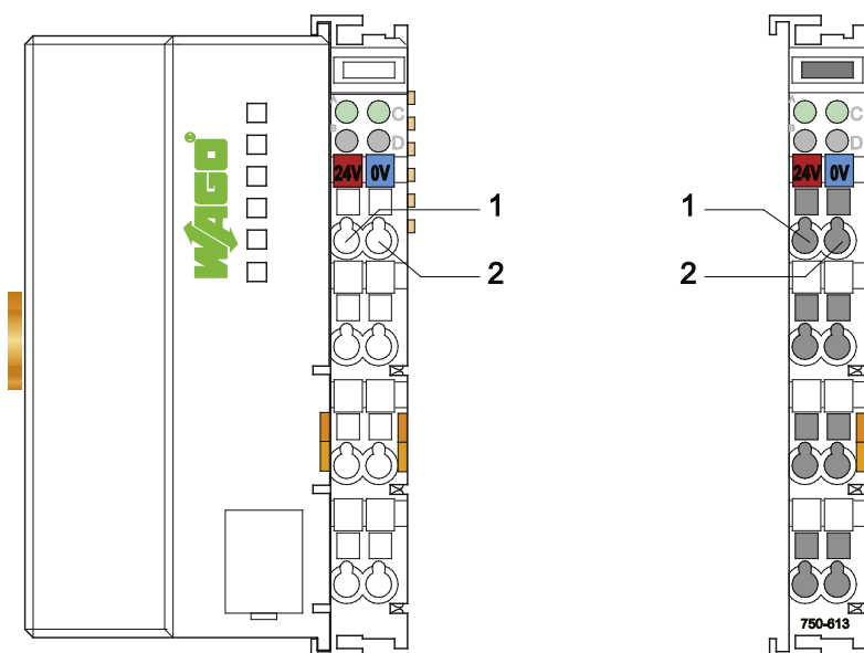
Figure 4: System Supply via Fieldbus Coupler/Controller (left) and via Internal System Supply Module (right)
