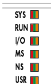
Figure 51: Indicating elements for fieldbus/system
