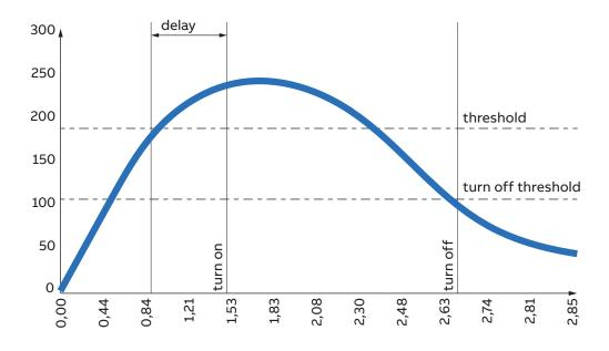
**How the alarm is turned on:** Whenever measured value crosses threshold for a time that is higher than the defined delay, timer is set and starts counting down delay. If count down is finished and the value have not crossed back the threshold, alarm is turned on. At this point, according to configuration, alarms trip is registered in the notifications log (alarm section) and/or alarm output is set High.
