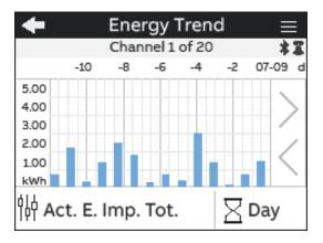
Move with \( \lambda \) keys to change the parameter. It is possible move among a list of channels, up to 20 parameters (Parameter Ch.1, Parameter Ch.2, etc...).
