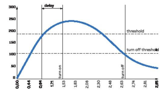
How the alarm is turned on: Whenever measured value crosses threshold for a time that is higher than the defined delay, timer is set and starts counting down delay. If count down is finished and the value have not crossed back the threshold, alarm is turned on. At this point, according to configuration, alarms trip is registered in the notifications log (alarm section) and/or alarm output is set High.
