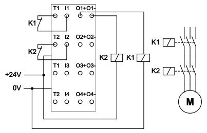
Figure 18: Load between Ox+ and 0 V, as well as 24 V and Ox-
