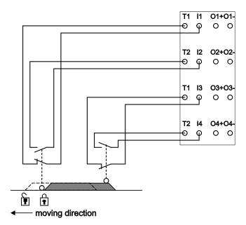
Figure 28: Connection 1 x Interlock Monitoring, Dual Channel, Antivalent Evaluation
