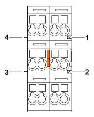
Figure 6: Power Jumper Contacts
