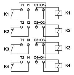
Figure 15: Load Between Ox+ and Ox-
