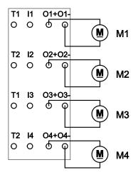
Figure 35: 4 x DC Motor Connection
