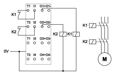
Figure 16: Load Bbtween Ox+ and 0 V
