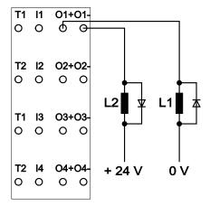
Figure 4: Connection Variant with 2 Diode Recovery Circuits
