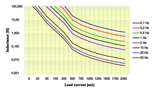
Figure 2: Switching Frequency Based on the Inductance and Load Current
