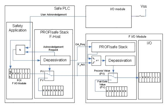
Figure 38: Schematic Representation for User Acknowledgement via "OA\_Req" and "F\_Ack"
