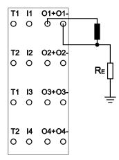
Figure 1: Grounded Load Connection
