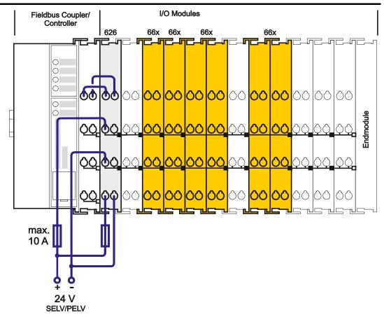
Figure 23: Infeed for F I/O Modules 750-66x and 753-66x
