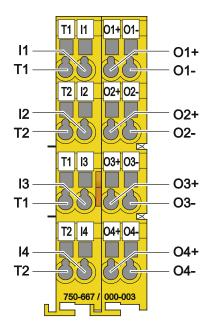
Figure 7: CAGE CLAMP® Connectors
