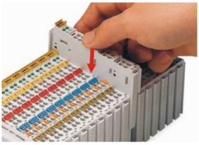
Figure 20: Snap the I/O Module into Place (Example)
