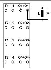
Figure 3: Connection Variant with Diode Recovery Circuit
