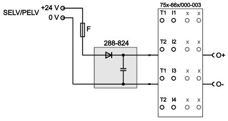
Figure 24: Infeed for PROFIsafe I/O Modules 75x-66x with Backup Capacitor Module 288-824
