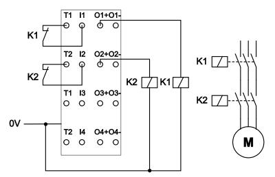
Figure 32: Connecting Loads from Ox+ to Ground Connection 0 V
