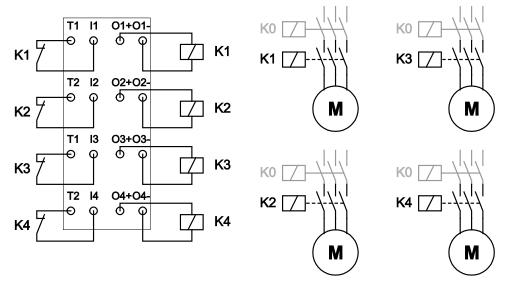
Figure 33: 4 x Motor Connection, Single-Channel with Feedback
