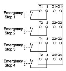
Figure 25: Connection 4 x Emergency-Off, Single-Channel, Short-Circuit Test Active
