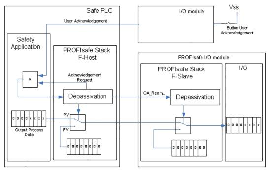
Figure 37: Schematic Representation for User Acknowledgement via "OA\_Req"
