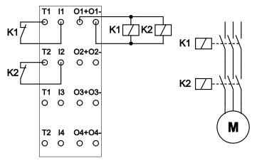
Figure 31: Connecting Two Parallel Loads to a Digital Power Output
