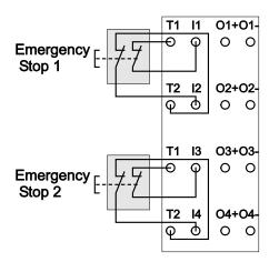
Figure 27: Connection 2 x Emergency-Off Switch, Dual Channel, Equivalent Evaluation
