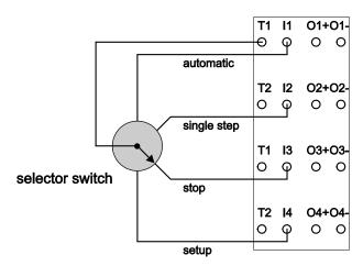
Figure 29: Connection 1 x Mode Selector Switch
