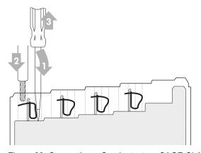
Figure 22: Connecting a Conductor to a CAGE CLAMP®
