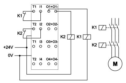
Figure 30: Connecting Loads from Ox+ and Ox- to 0 V and 24 V
