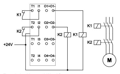
Figure 17: Load between 24 V and Ox-
