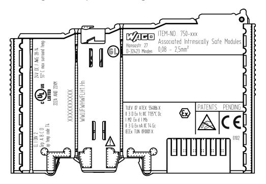
Figure 39: Marking Example According to ATEX and IECEx
