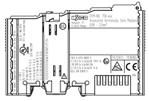
Figure 41: Marking Example for Approved I/O Module Ex i According to ATEX and IECEx
