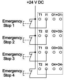
Figure 26: Connection 4 x Emergency-Off, Single-Channel, Short-Circuit Test Not Active
