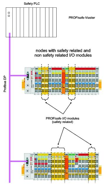
Figure 1: Mixed Operation of Safety-Related and Non-Safety-Related I/O Modules
