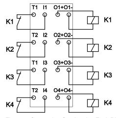
Figure 5: Connecting One Load to Each Digital Power Output
