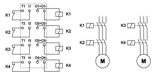
Figure 34: 2 x Motor Connection, Two-Channel with Feedback
