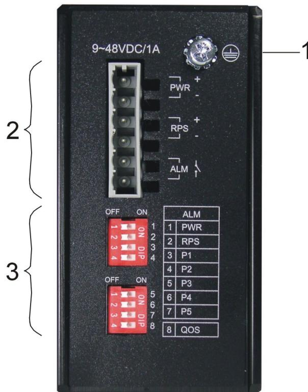
Figure 2: Top View of the Industrial Switch
