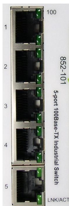
Figure 7: Port LEDs
