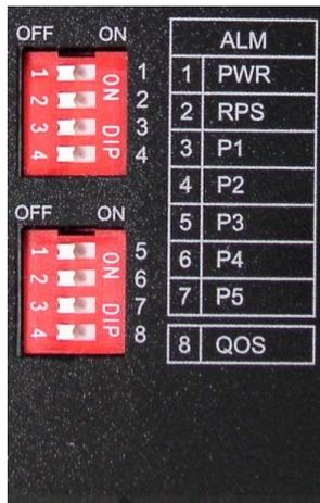
Figure 8: DIP Switches
