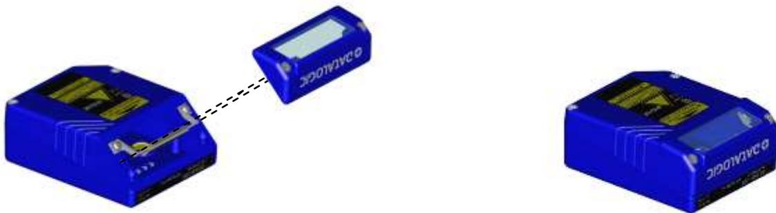
Figure 19 - Mounting a GFC-2020 Deflection Mirror
