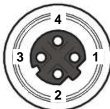
Figure 97 - M12 D-Coded 4-pin Female Profinet-IO Network Connector
