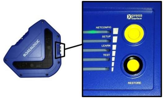
Figure 43: Control Panel Buttons
