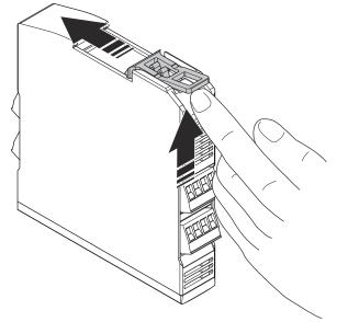
Figure 59: Reset the DIN rail latching device.
