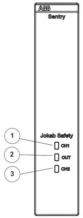
Figure 46: Indication LEDs on BSR23
