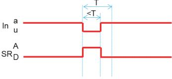
Figure 53: Stopped timer reset function
