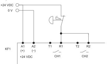
Figure 34: 1 channel connection, +24 VDC static signal
