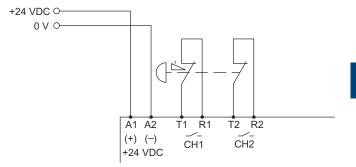
Figure 37: 2 channels connection with equivalent contacts from T1/T2  $\,$
