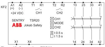
Figure 15: Connections TSR20
