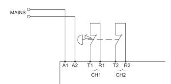
Figure 38: 2 channels connection with equivalent contacts from T1/T2
