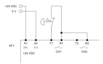
Figure 35: 1 channel connection from T1
