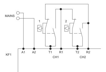
Figure 44: Two-hand safety device connection with square wave signal (SSR20M)
