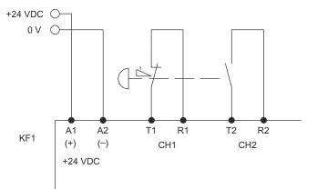
Figure 40: 2 channels connection with antivalent contacts from T1/T2  $\ensuremath{\mathsf{T1}}$
