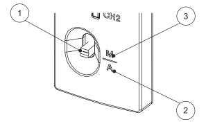
Figure 61: Switch for automatic reset and manual reset.
