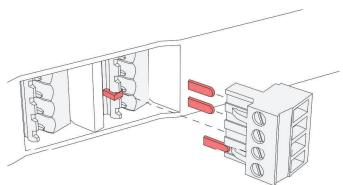
Figure 60: Example of connection block coding
