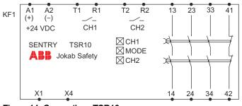
Figure 14: Connections TSR10
