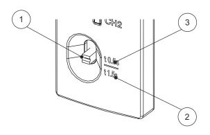
Figure 62: Switch for Off-delay settings.
