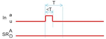
Figure 49: The safety input goes low within the delay time
