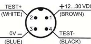
\* in case of white wire or pin 2 not connected the sensor operates in LIGHT mode for the proximity models (S15...Cxx/D50/M01) and in DARK mode for the retroreflex (S15...A0x/B0x/T01) and receiver models (S15...F0x).
