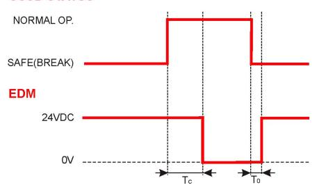
$T_C \ge 350$  msec: 350 msec: time after OSSD OFF-ON switch when EDM test is performed.
