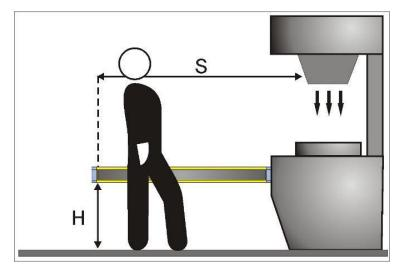
Fig. 4 - Minimum installation distance (horizontal)
