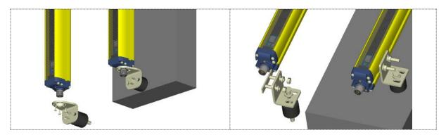
Fig. 19 – Mounting rotating brackets
