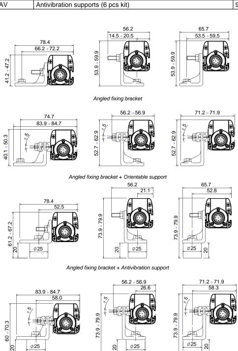
Angled fixing bracket + Orientable support + Antivibration support
