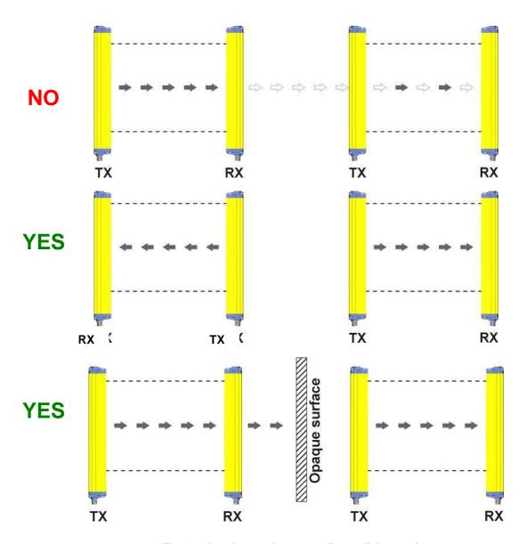
Fig. 13 - Interference between adjacent light curtains
