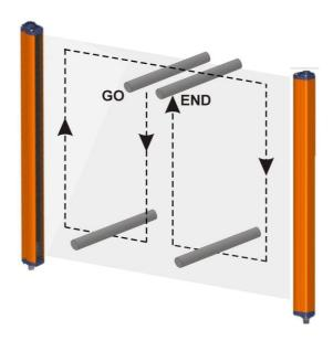
Fig. 16 - Path of the test piece
