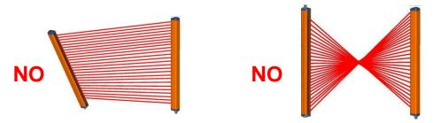
Fig. 14 - Light curtains orientation
