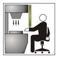
Fig. 5 - Incorrect device positioning
