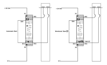
Fig.21 - Connection to safety relay
