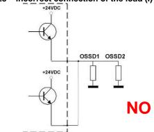
Fig. 24 - Incorrect connection of the load (II)
