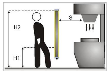
Fig. 3 - Minimum installation distance (vertical)
