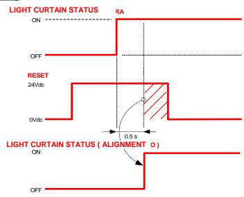
Once optimal alignment has been reached, the device can return to normal functioning by powering off and then powering on the RX unit.
