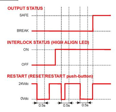
Select either automatic or manual restart by connecting pin of RX connector (see section 4 "Electrical connections")
