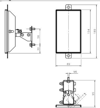
The image includes the mirror SG-DM and a mounting kit ST-DM.
