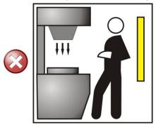
Fig 11 - Wrong light curtain positioning
