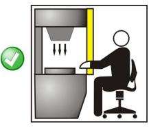
Fig 10 - Correct light curtain positioning
