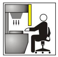
Fig 9 - Wrong light curtain positioning
