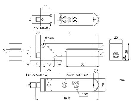
To install the sensor using the connector positioned at 90°, unscrew the blocking screw and rotate the fixing block in an anti-clockwise direction. At the end rescrew the blocking screw.
