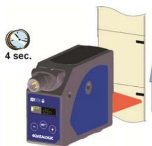
If the detection has been successful, the sensor returns to normal functioning. If it fails due to insufficient contrast, the 'Lo' test blinks on the display. Press the (SET) push-button to repeat procedure until releasing the button (the 'dYn' text blinks on the display). The sensor returns to the previous setting by pressing (+) or (-).
