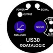
The sensor may be programmed either via ANALOG push-button, or via a remote command (remote teach). Remote programming may be used to disable the push-button, preventing unauthorized personnel from adjusting the programming settings. To access this feature, connect the Remote Teach wire of the sensor to 0 Vdc, with a remote configuration switch between the sensor and the voltage.
