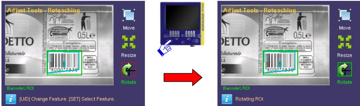
To rotate the ROI, select the **“Rotate”** option from the Setup menu (using the **SET** button again). The ROI will rotate in a clockwise/anticlockwise directly depending of the **RIGHT/LEFT ARROW** button pressed.
