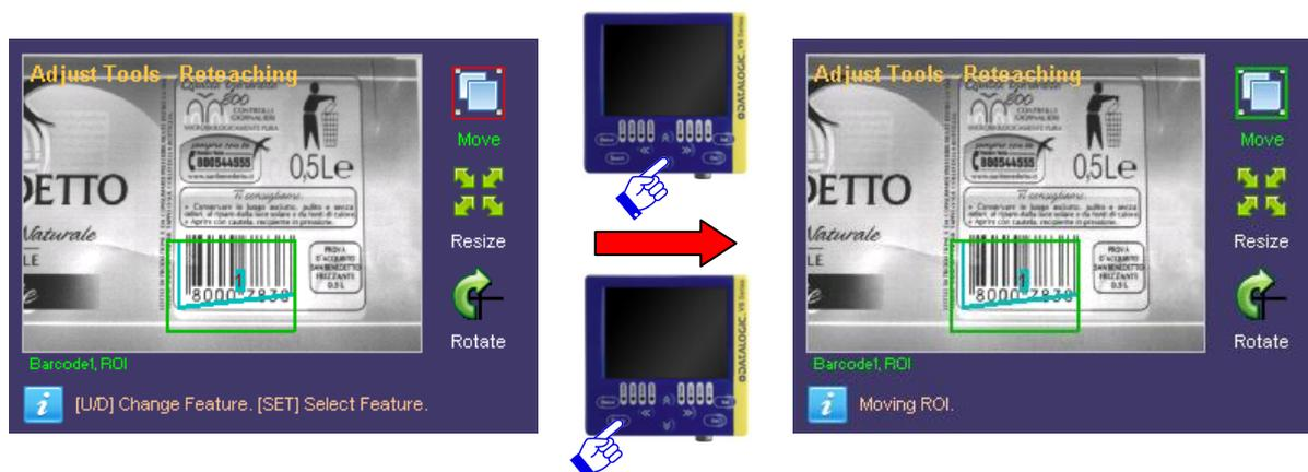
Once selected **“Move”**, the focus is transferred in the field range and the ROI can be moved using the **ARROWS**. Once you have achieved the desired position, press **TEACH** to save changes. Press **ESC** to return to the Setup menu ignoring the changes made.
