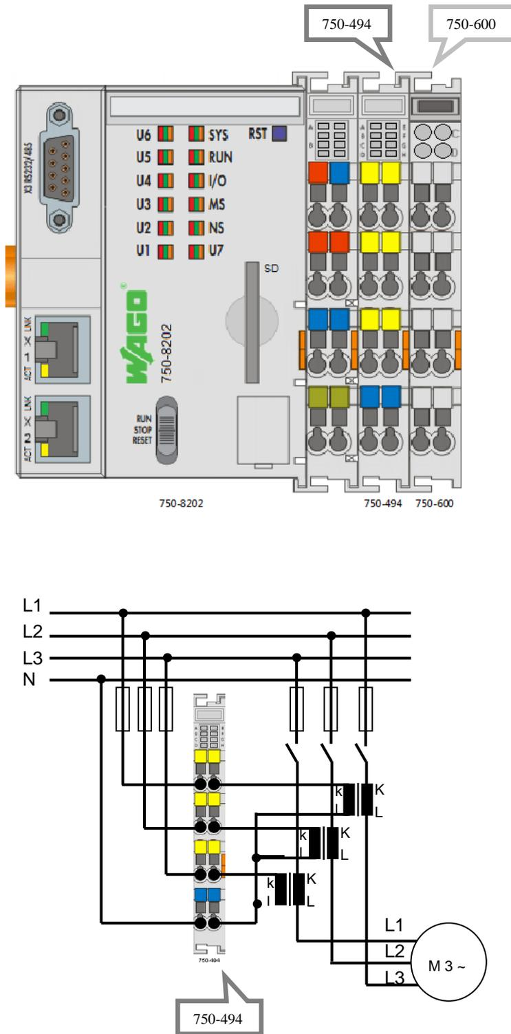
Figure 1: Connection diagram
