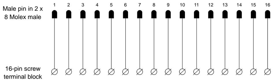
Note: 16-pin screw terminal block with internal connection adapted for a common monitoring unit. Designed for a manually connected cable. Anti-cheat-board is an option.
