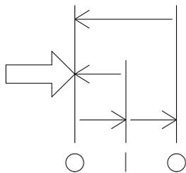
The symbol for the 3-position switch shows the three positions (OFF, ON, OFF) with O and I, actuating force from left to right, and possible paths for the switch (IEC 60947-5-8:2006).
