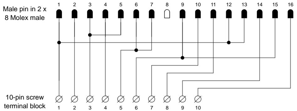
\* Note: The COM signal must be +24 VDC to allow the LEDs and anti-cheat-board to function properly.
