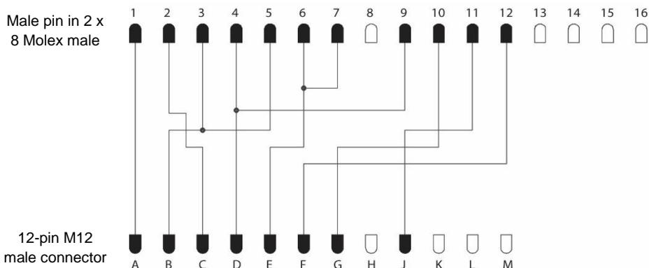
\* Note: The COM signal must be +24 VDC to allow the LEDs to function properly.
