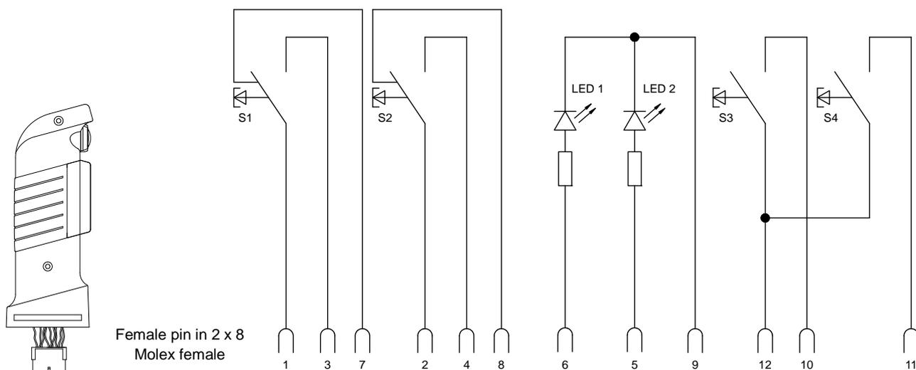
Note: 2 x 8 Molex females on the top parts JSHD4-2...5 fit into the corresponding connector on the bottom parts.
