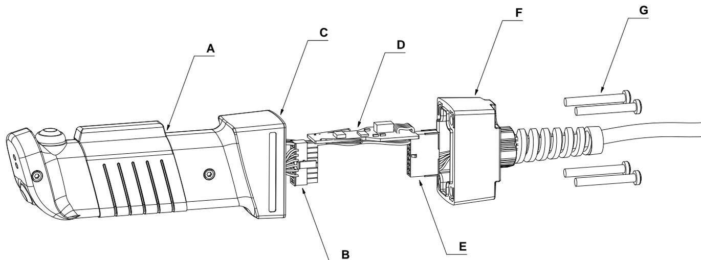
1. If available, connect the pins from the anti-cheat-board (D) to connector (B) on handle (A).
