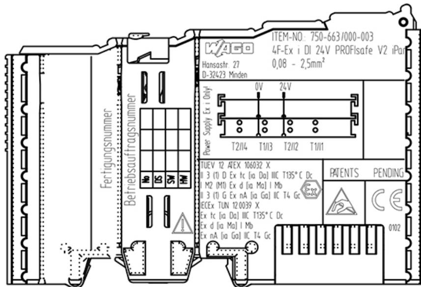
Figure 16: Side Marking Example for Approved Ex i I/O Modules According to ATEX and IECEx.
