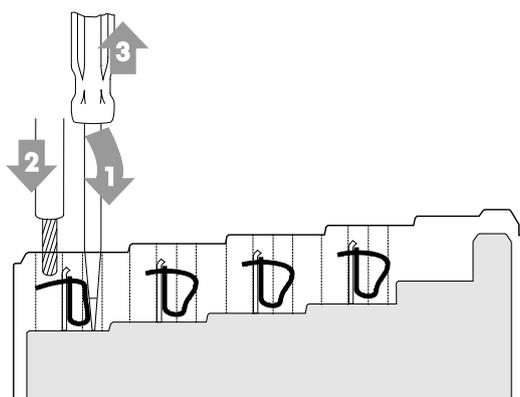
Figure 10: Connecting a Conductor to a CAGE CLAMP®
