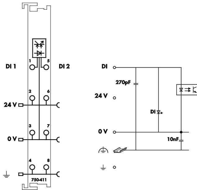
Figure 6: Schematic Diagram
