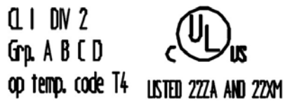
Figure 23: Printing on text detail in accordance with NEC
