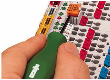
Figure 8: Removing the Fuse Carrier
