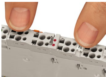
Figure 15: Plugging the Connector into Place
