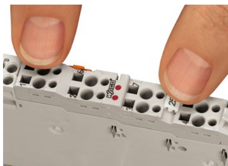
Figure 15: Plugging the Connector into Place
