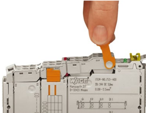
Figure 17: Pulling the Pull Tab
