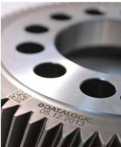
High contrast marking on metal
