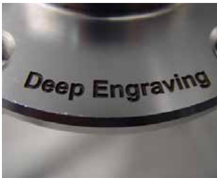
Engraving & deep engraving on metal
