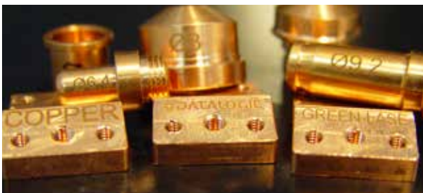
Green: marking on copper
