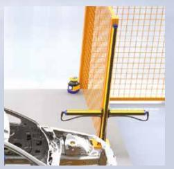
Areas around the car body are monitored using LASER SENTINEL safety laser scanner. Thanks to protective field of 5,5m, only two scanners are required for full protection of the work area. By using Master Slave connection, two scanners can be used together with a single point of programming and monitoring, and saving wiring and safety I/Os.
