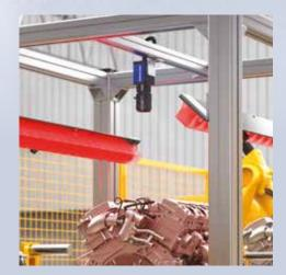
The MX-E Vision Processor Series, powered by the IMPACT Software suite with 100+ advanced inspection tools, supports multiple individual cameras, allowing either to inspect complex items like engine blocks leveraging multiple points of view or to deploy several verification points along the manufacturing line.
