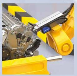
Quality standards along the production processes require accurate check points of the assembling phases. LD46 luminescence sensor is used to verify if the correct amount of adhesive layer has been applied on the edge of the engine head cylinders.
