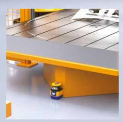
The LASER SENTINEL safety laser scanner for area monitoring prevents the start of a dangerous movement when someone is standing behind the light curtain. Automatic restart is possible when the hazardous area is empty.
