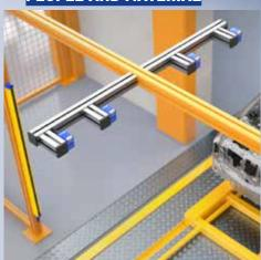
In the course of the production process, the bodies are lifted or lowered to different transport levels. The SG4 EXTENDED safety light curtain prevents entry of a person into the hazardous area.
