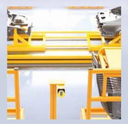
The safety laser scanner can monitor vertical openings through which people could enter into dangerous areas. Checking continuously the position of reference points, LASER SENTINEL guarantees that in case of mechanical changes, the dangerous movement could be stopped.
