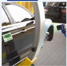
Automated assembling processes always require the identification of the car to ensure maximum quality and total production traceability. The Matrix 410N, featuring C-Mount lenses and powerful embedded illuminators, delivers robust barcode reading capabilities while covering a wide area.
