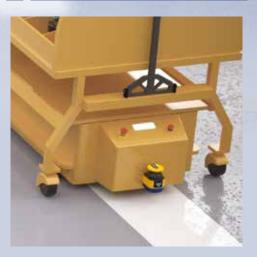
A LASER SENTINEL safety laser scanner can be used to protect the AGV against collision with persons, vehicles and material. The configurable protective and warning fields are activated dynamically according to the speed or curve traveled.
