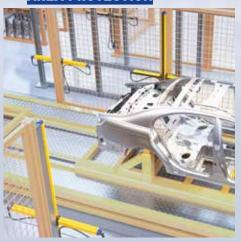
SG4 EXTENDED safety light curtains are used to separate cells in the paint line. Basic and Advanced configurations, for example partial muting on different areas, are possible through push buttons or Graphical User Interface.
