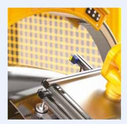
Windscreen assembling requires an accurate approaching phase of the robot gripper in order to guarantee a precise and soft positioning of it. The S85 distance sensor based on TOF technology is used to measure the approaching distance of the robot gripper from the body shop.
